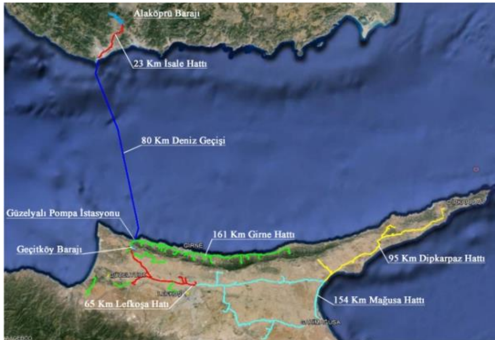
Figure 4. Map of the Water Supply Project (pipeline and distribution network). Source: DSI.
