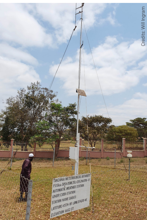
An automatic weather station in the grounds of Babati Town Council building, in Babati, Tanzania, operated by Tanzania Meteorological Authority.
