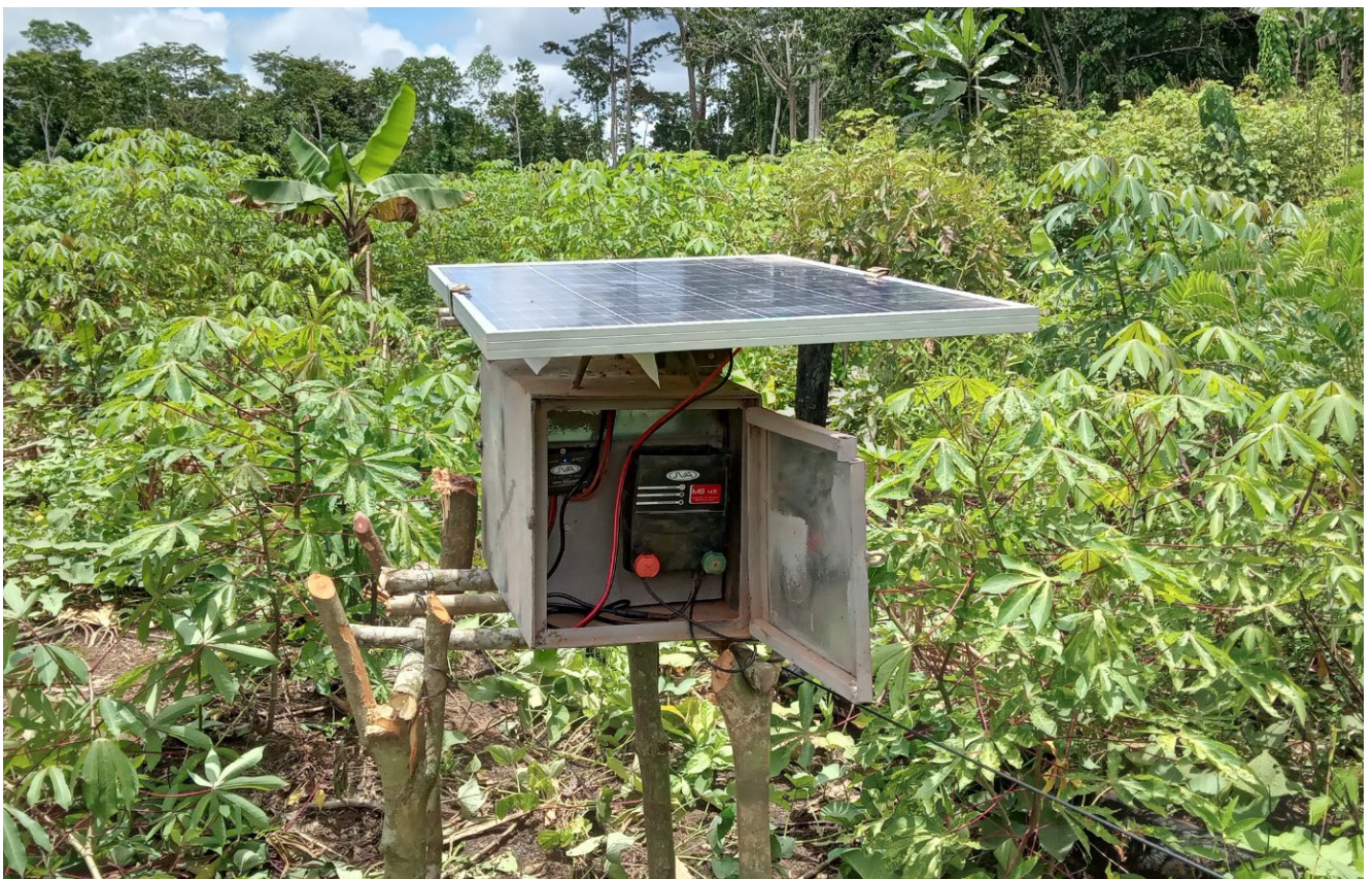
A solar-powered mobile electric fence unit, featuring a solar panel, battery, control box with wiring, and wooden posts for support. Photo: Space for Giants.
