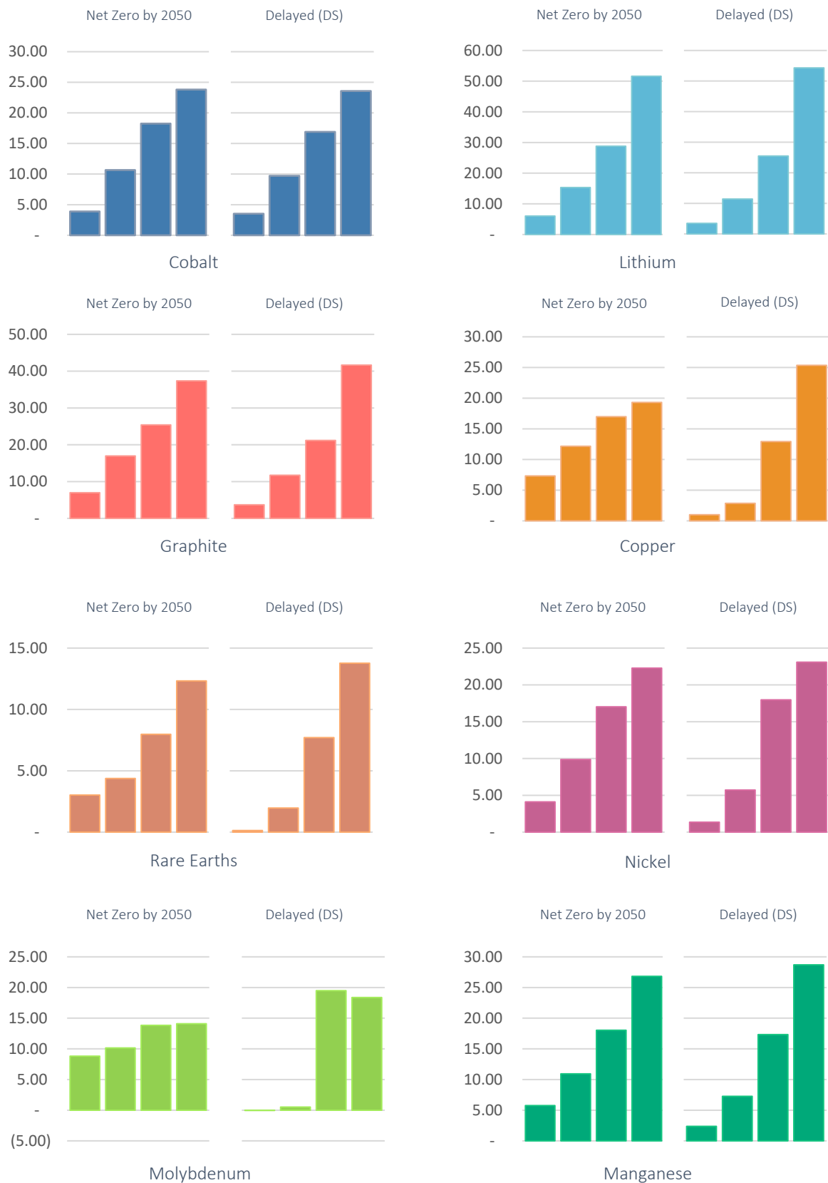
Figure 5. Material-specific relative demand growth for each five-year step average (2025, 2030, 2035, 2040) for both scenarios ('Net Zero by 2050' and 'Delayed Transition' scenarios), indexed to 2020
