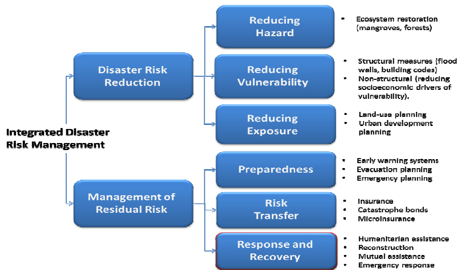
Figure 4. Schematic illustrating the components of an integrated disaster risk management strategy and examples of specific measures. Ex-post measures, implemented after a disaster, are circled in red.
