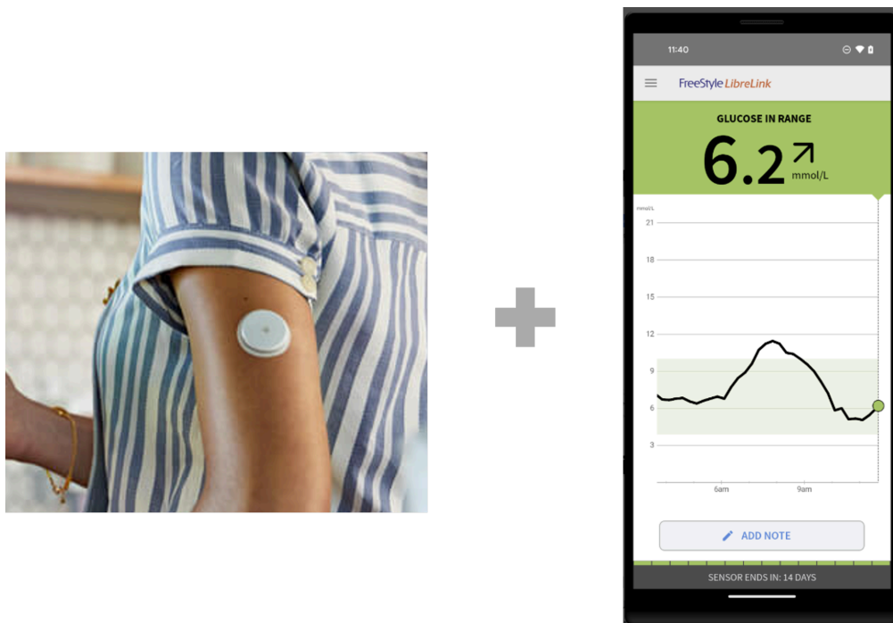
Figure 9. FreeStyle Libre 2 Continuous Glucose Monitoring (CGM) System: Sensor and associated smartphone application
