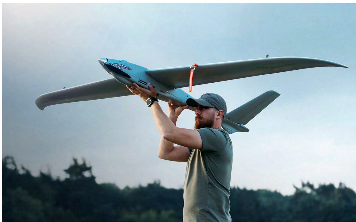
Preparing to launch a Mini Shark UAS fixed-reconnaissance drone produced by Ukrspesystems. Photo credit: Ukrspesystems.
