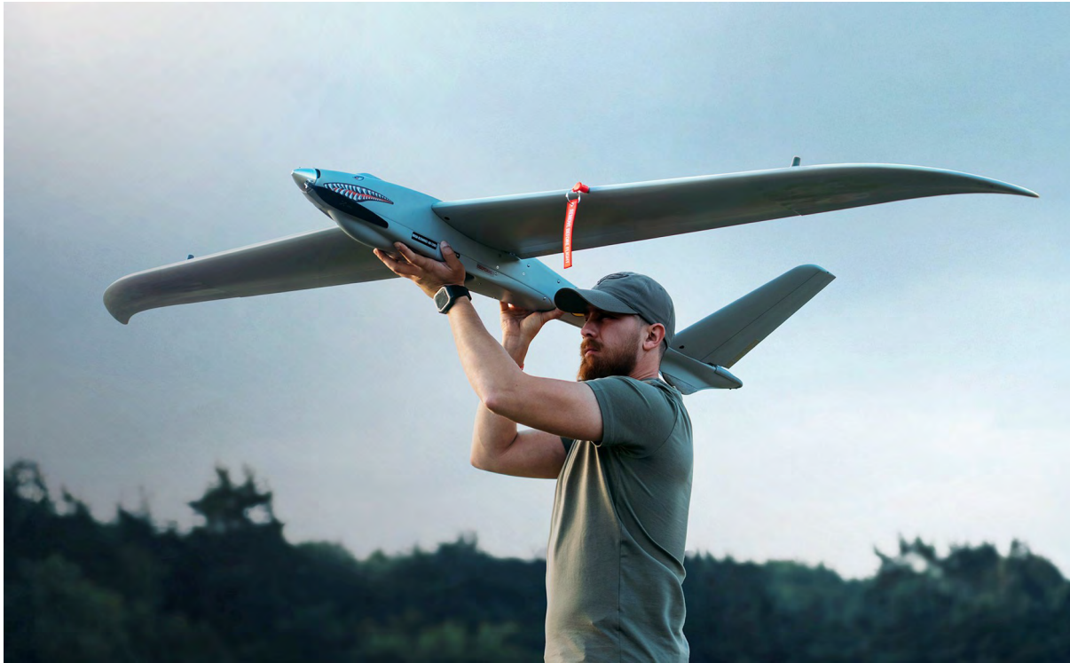
Preparing to launch a Mini Shark UAS fixed-reconnaissance drone produced by Ukrspesystems. Photo credit: Ukrspesystems.
