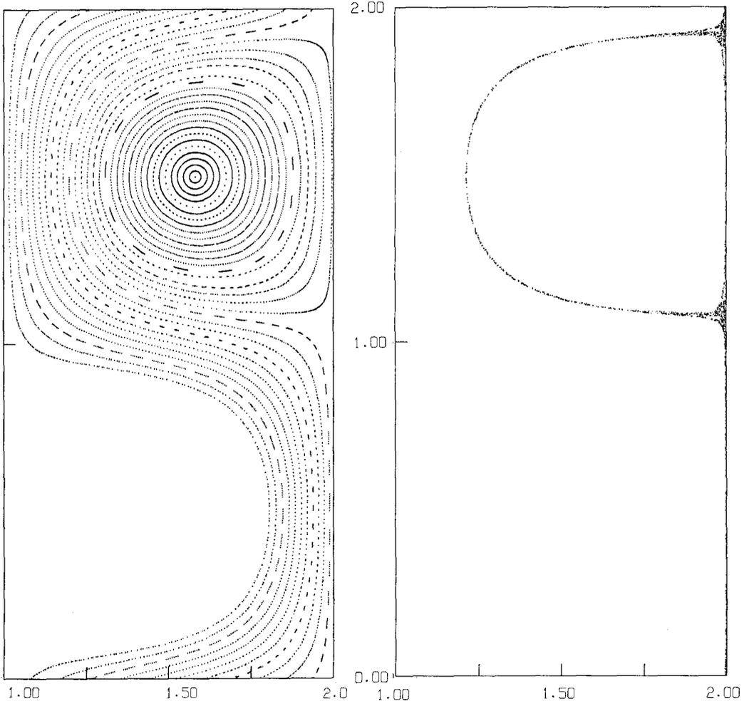
**Fig. 3.3.** Orbits with falling particles subjected to periodic boundary conditions and shown stroboscopically for  $\epsilon = 0.01$ ,  $\gamma = 0.25$ ,  $\omega = \pi/2.25$ . (a) For thirty-two particles starting out uniformly on  $y = 3/2$  and followed for 300 oscillation periods of the fluid flow. (b) For four particles starting out on  $y = 2$ , so as to be in the chaotic region, and followed for 500 periods.
