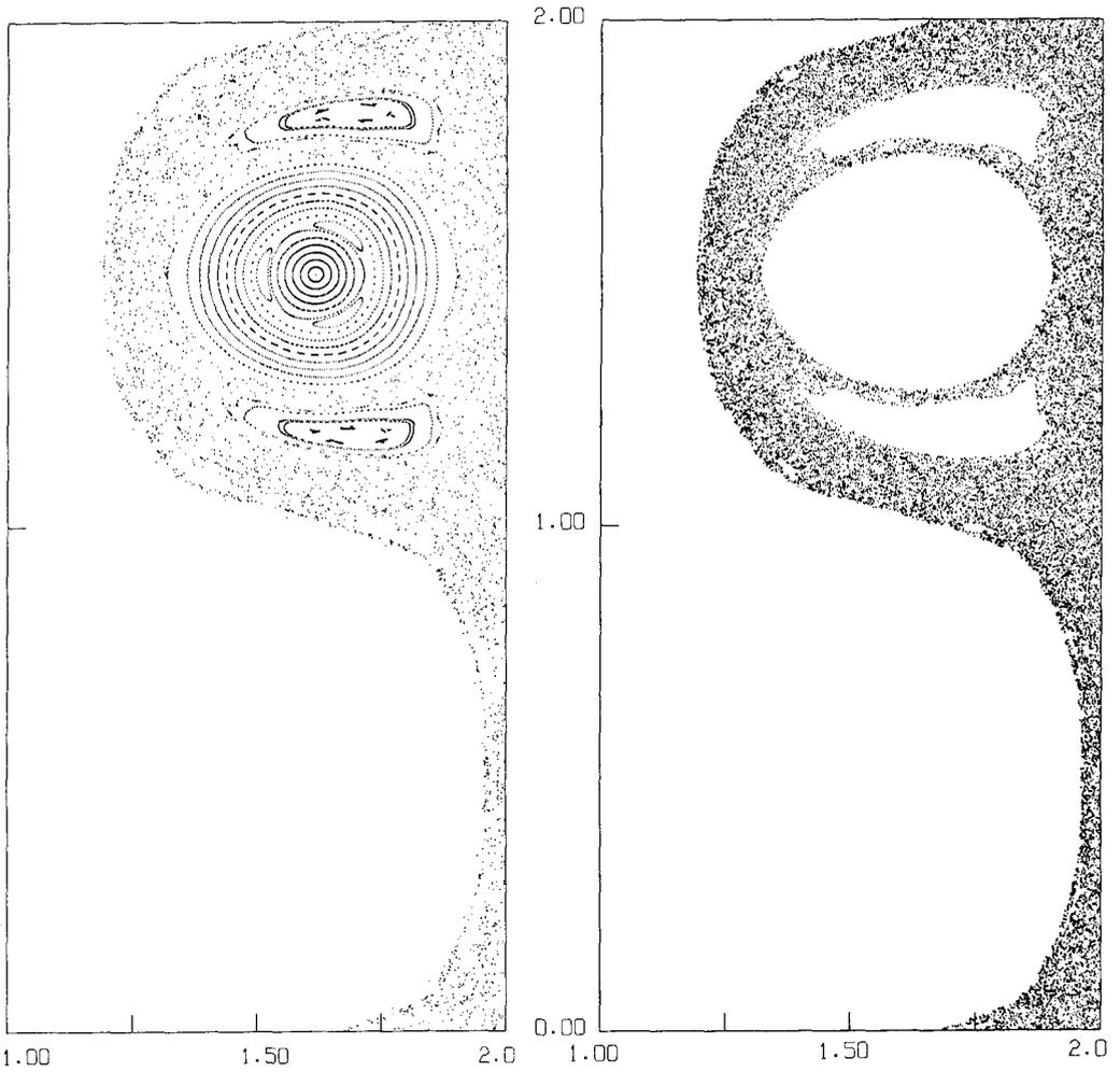
**Fig. 3.4.** Same as in Fig. 3.3 but with  $\epsilon=0.05$ . This time, the orbits in (a) have been followed for 400 oscillation periods and those in (b) for 3000. To the left edge of the chaotic region integrable orbits are found, though they are not shown in the figure.
