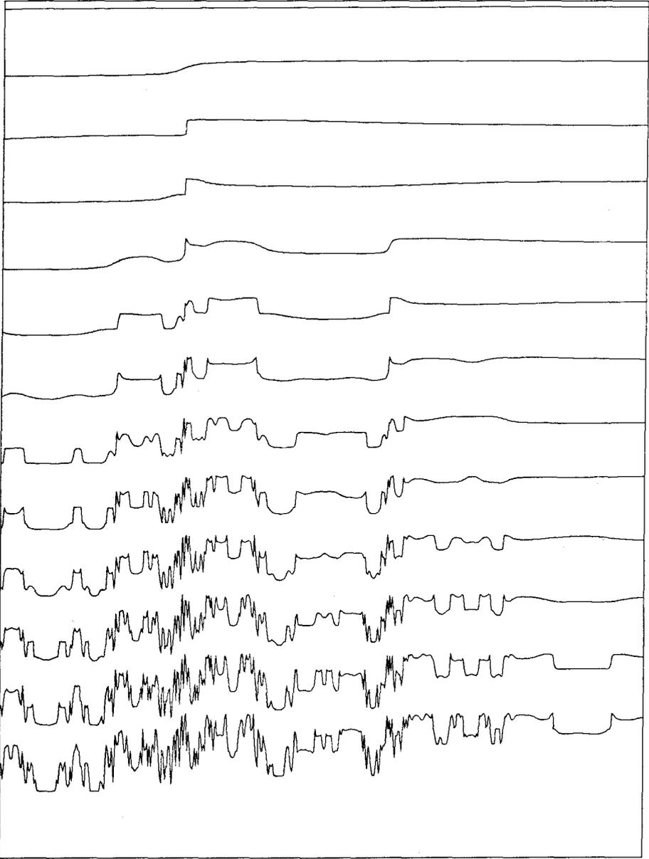
Fig. 3.7. The evolution of an initially simple particle distribution. Shown for a sequence of times separated by one period of oscillation of the fluid. The range in  $x$  is 0.0 to 0.1. The height of the box is 110 cell heights. The vertical offset of each curve is linear with time.
