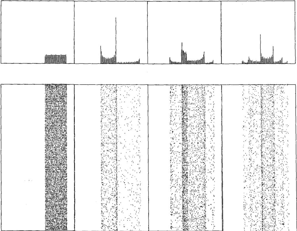
Fig. 2.3. The particle densities integrated (in  $y$ ) for the four states of Fig. 2.2. The upper panels show the particle number explicitly and the lower panels are 'dust plots' simulating the appearance of the convected dust.
