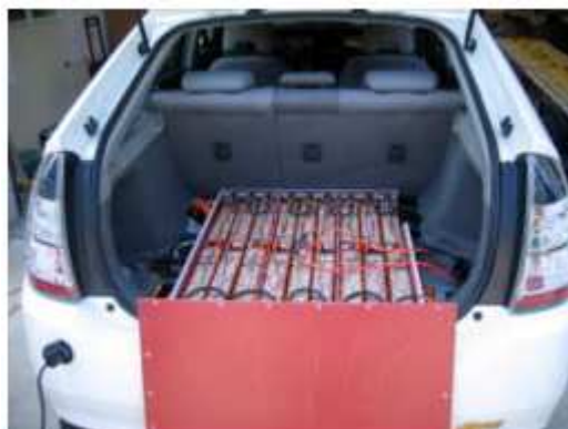
Figure 11 - Conversion to plug-in hybrid using Lithium-ion battery pack
