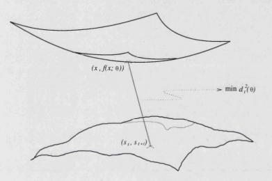
Figure 4.4: The TLS cost function is the minimum average distance between the surface defined by the observation pairs,  $(s_t, s_{t+1})$ , and a point in the model hypersurface,  $(x, f(; \theta))$ . For each pair and fixed value of  $\theta$ , a value of x is found such that  $d_t^2(x; \theta)$  is minimum.
