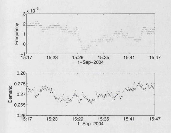
Figure 6.1: Trace of a 30 min. on  $1^{st}$  September 2004 between 15:17 to 15:47. The grid frequency plotted in the upper panel is the fractional deviation from the operational point of the grid system  $\omega_0$  and the demand plotted in the lower panel is normalised with respect to the total load of the grid  $\mathcal{G}$ .
