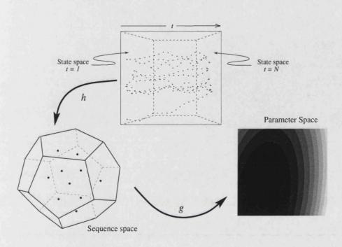
Figure 4.1: The diagram represents how the information form the dynamics and the observations is carried for particular values of the parameter vector  $\boldsymbol{\theta}$  to the sequence state and finally to the parameter space via some mapping of relevant statistics represented by g.
