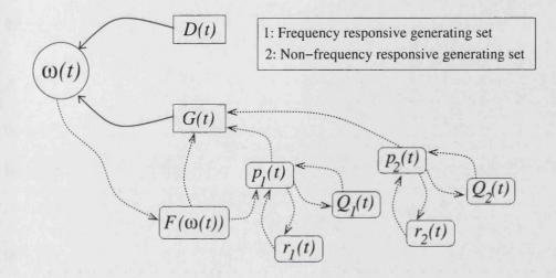
Figure 6.3: The diagram shows the dependency relations between the grid frequency and the internal variables of the model. Arrows pointing to a node, *i.e.* circles, squares or rounded squares, come from variables on which the node depends explicitly.
