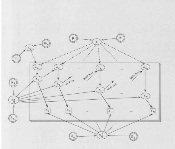
Figure 3.1: DAG for the Logistic map probability model structure. Squares represent model observables, circles non-observables, *i.e.* the model parameters, and double circles hyper-parameters included to model the probability model parameters. Dashed lines represent deterministic relations while solid lines stand for probabilistic dependency. The layered panels represent algorithmic iterations.
