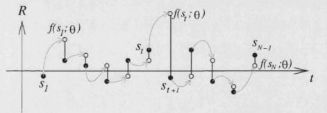
Figure 4.2: The LS cost function is the one-step prediction error. The black dots represent the observations, the white filled circles the iteration of the map  $f(\cdot)$  from the observation  $s_t$  and the vertical lines are the distances  $d_t^2(\theta)$  that defined  $C_{LS}(\theta)$  for a given trajectory segment.
