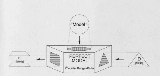
Figure 6.4: Sketch of the forward simulation for the grid frequency model. The synthetic demand data (pyramid in the right) drives the numerical integration of the model to obtained grid frequency (box in the left).
